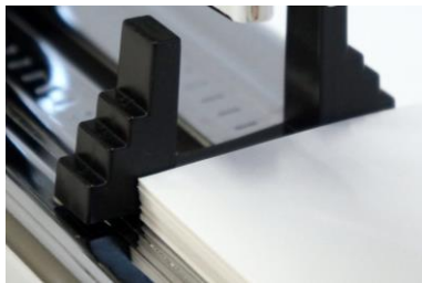
Adjustable paper stopper with thickness ruler
